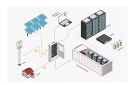
Jun 24, 2025 · What is a photovoltaic inverter? A photovoltaic inverter is an electronic device that converts the direct current (DC) generated by solar panels into alternating current (AC). Only ...
