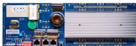
RS485 Communication between battery and inverter Band rate 9600bps RS485 Interface Communication between parallel packs or BMS and PC Band rate 9600bps
